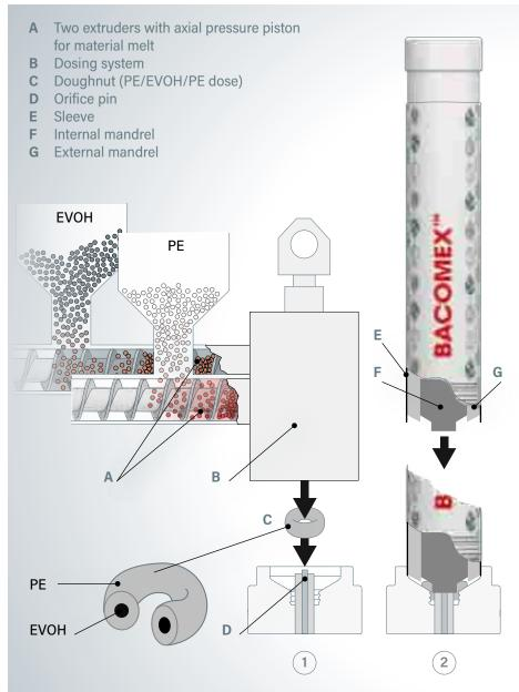
1 A controlled flow under pressure traps the EVOH barrier in the middle of the PE donought. 2 Outer and inner parts (F)(G) of the mandrel are pushed down. The outer part (G) of the mandrel is closing the mould before pressure is applied.
