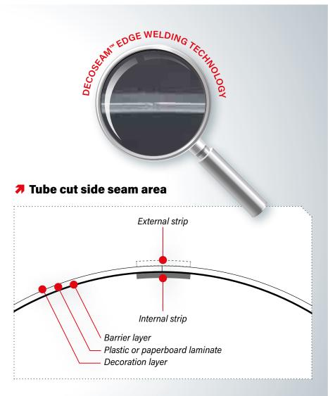
To prevent the paperboard from absorbing external moisture, a second strip is welded on the outside of the sleeve.
