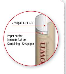
DIBS - Double Induction Belt Sealing for both Aluminium and Plastic Barrier Laminate (ABL & PBL)
