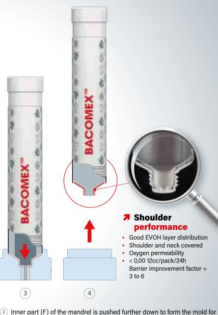
③ Inner part (F) of the mandrel is pushed further down to form the mold for the tube head. ④ The mandrel lifts up, the shoulder is perfectly moulded and welded with a clean orifice to the sleeve. The multi-layer barrier is formed during the compression moulding.
