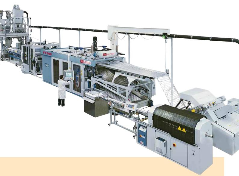
All FT machines can be supplied as an in-Line series, forming a real "production island" starting from the raw material up to the finished product, including the IN-LINE recycling of the granulated scrap.
