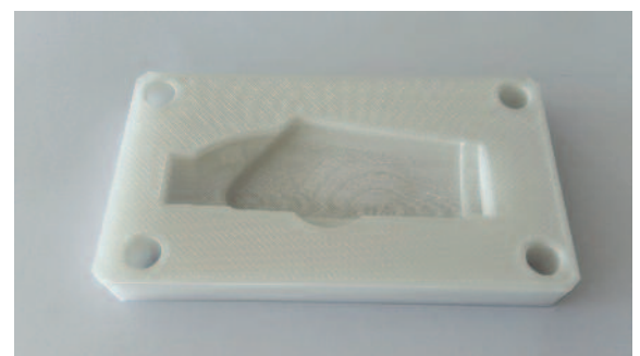
Bio-compatible POKA YOKE device in lightweight construction
