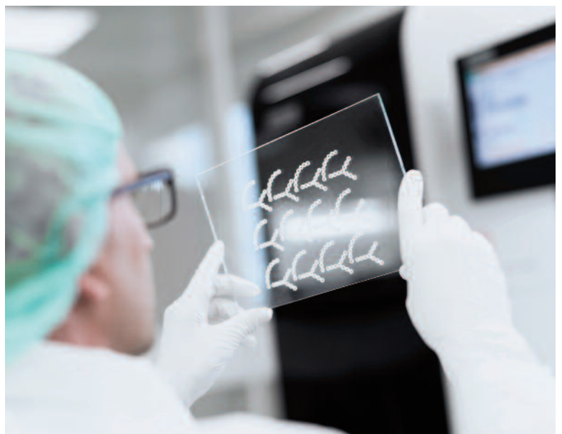
Glass plate as carrier material for Freeforming of resorbable C and Y plates
