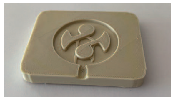
PEEK mould insert for an injection mould
