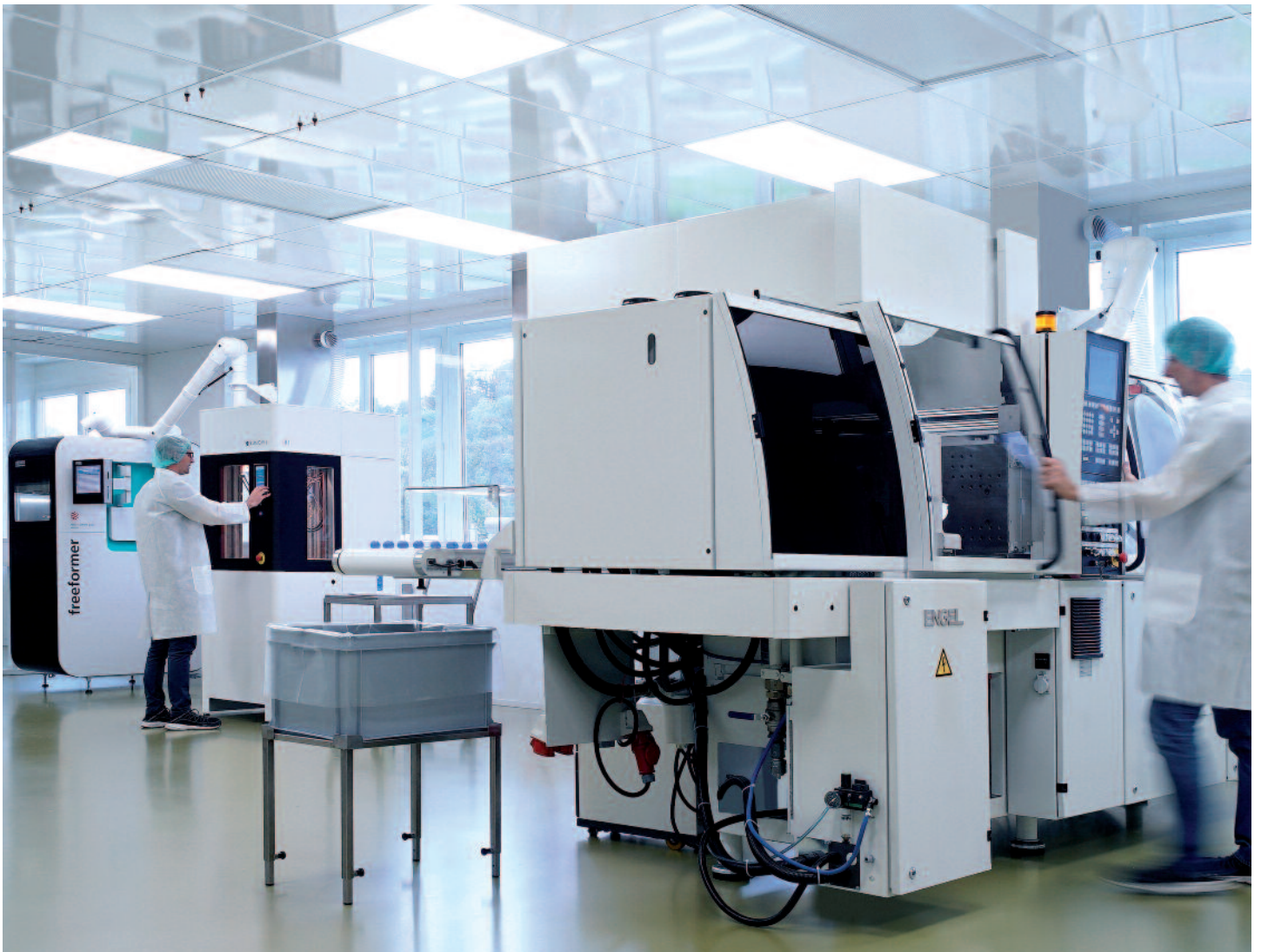
Additive Manufacturing in clean room (ISO 8) in a qualified environment
