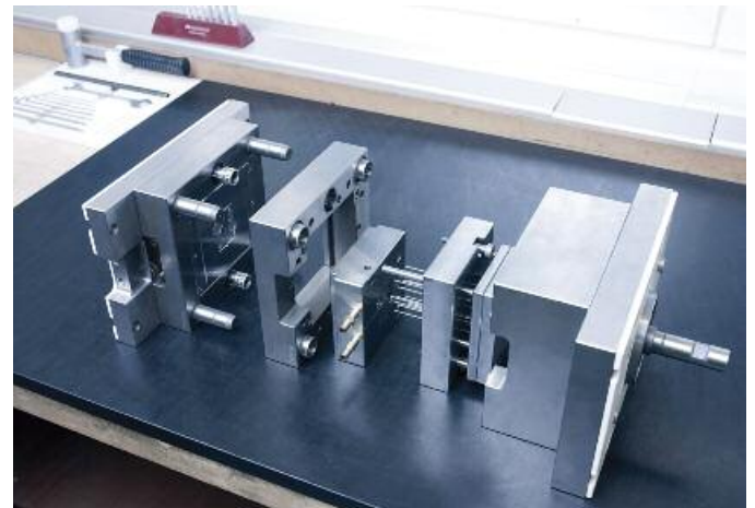
Figure 13: Interchangeable inserts/modular form (master form)
