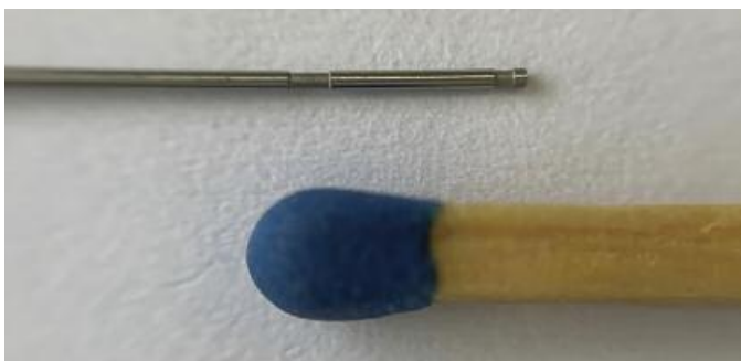
Figure 16: Rotating cutting with indexing at \varnothing 0.4 mm with accuracy of 0.002mm
