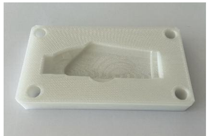
Figure 9: POKA-YOKE fixture made with AM
