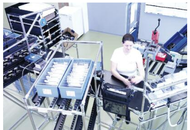
Figure 34: Assembly in One-Piece Flow (LEAN)
