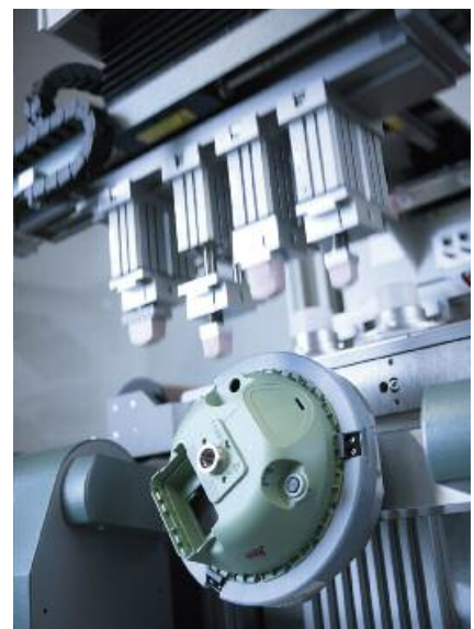
Figure 31: Pad printing robot (automation)
