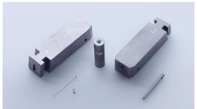
Figure 12: Micro insert - for resorbable screws M1.5
