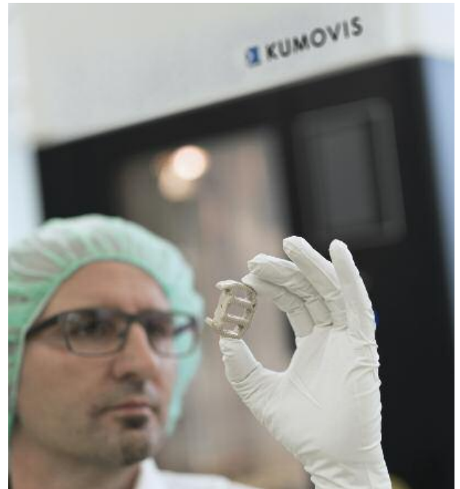
Figure 26: Peek cages produced with AM
