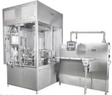
Dosing range: 125-500 ml Maximum output: up to 105 packs/min
