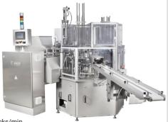
Dosing range: 200-1000 g Maximum output: up to 40 packs/min Dimensions: (L x W x H) ~ 4260 x 2455 x 1900 mm
