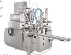
Dosing range: 135-240 ml Maximum output: up to 50 packs/min Dimensions: (L x W x H) ~ 3170 x 1470 x 1540 mm
