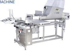
Dosing range: 5, 10, 15, 20, 25 kg Maximum output: up to 151 cartons/h Dimensions: (L x W x H) ~ 2405 x 1360 x 1282 mm
