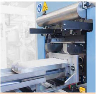
Thermoforming Machine TWIST 300 works with air pressure and simultaneous in-mould punching, vertical movement and 90° rotation of the lower platen.
