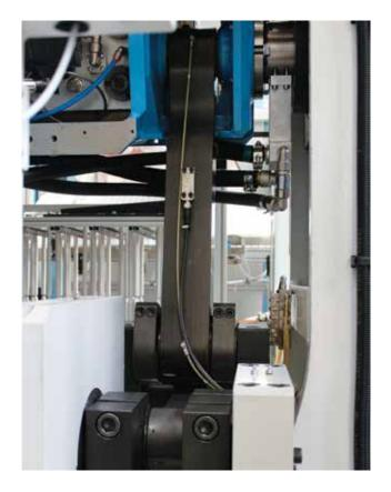
The lower tilting platen, moved without mechanical cams, rotates 75° and is guided on prismatic linear guides to reduce vibrations.
