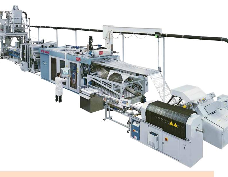
TWIST 700 machines can be supplied as an IN-LINE series, forming a real "production island" starting from the raw material up to the finished product, including the IN-LINE recycling of the granulated scrap.
