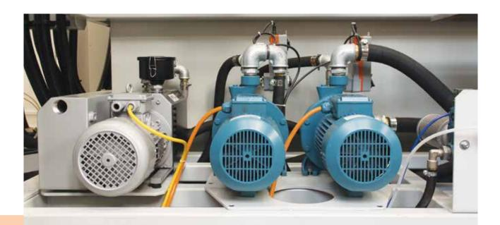
The TWIST 700 has integrated two independent mould temperature circuits to keep constant the  $\Delta T$  in 2°C between the upper and lower mould.
