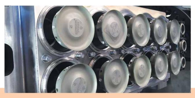
Electric extractor for better cycle synchronization is not requiring any mechanical stopper inside the mould, therefore reducing overall maintenance.
